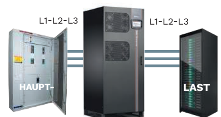
3-adrige Installation (L1-L2-L3)
